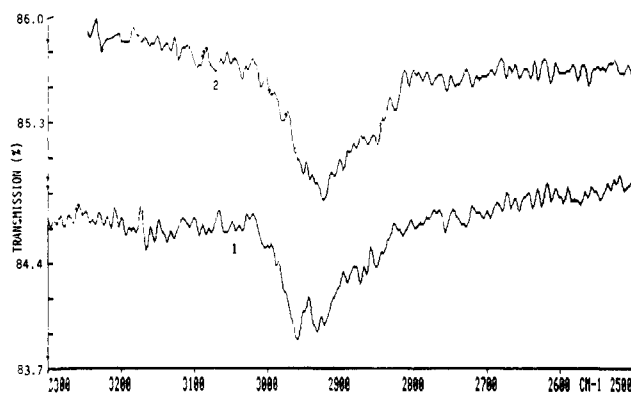
Figure 4. Expansion of the 3300–2500- \text{cm}^{-1} region in the FT-IR spectra in Figure 3 to illustrate the differences in the intensity of the C–H absorption at 2960 and 2870 \text{cm}^{-1} .
